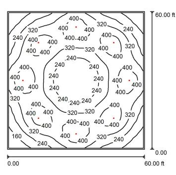
Height of Room: 18.000 ft, Mounting Height: 18.000 ft, Light loss factor: Values in Lux, Scale 1:250 0.80
